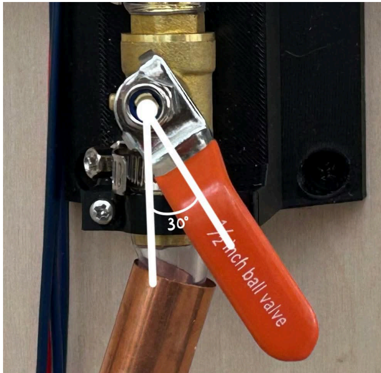
Figure 7.3.1: Minimum Angle of Lever of Valve 4 to Trigger Leak State.
