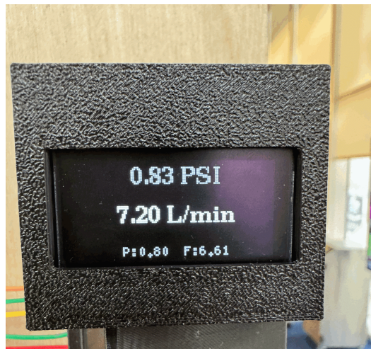
Figure 7.2.1: OLED Screen on Hardware System Displaying Live Sensor Values.
