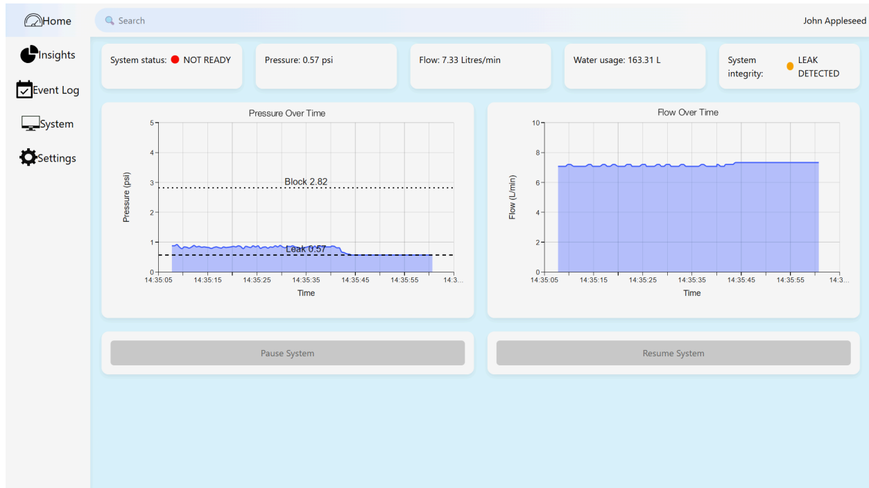
Figure 7.1.1: Dashboard Alerted of Leak Detected State.
